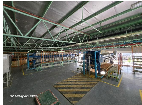
Degrease Wastewater Treatment System UT1
